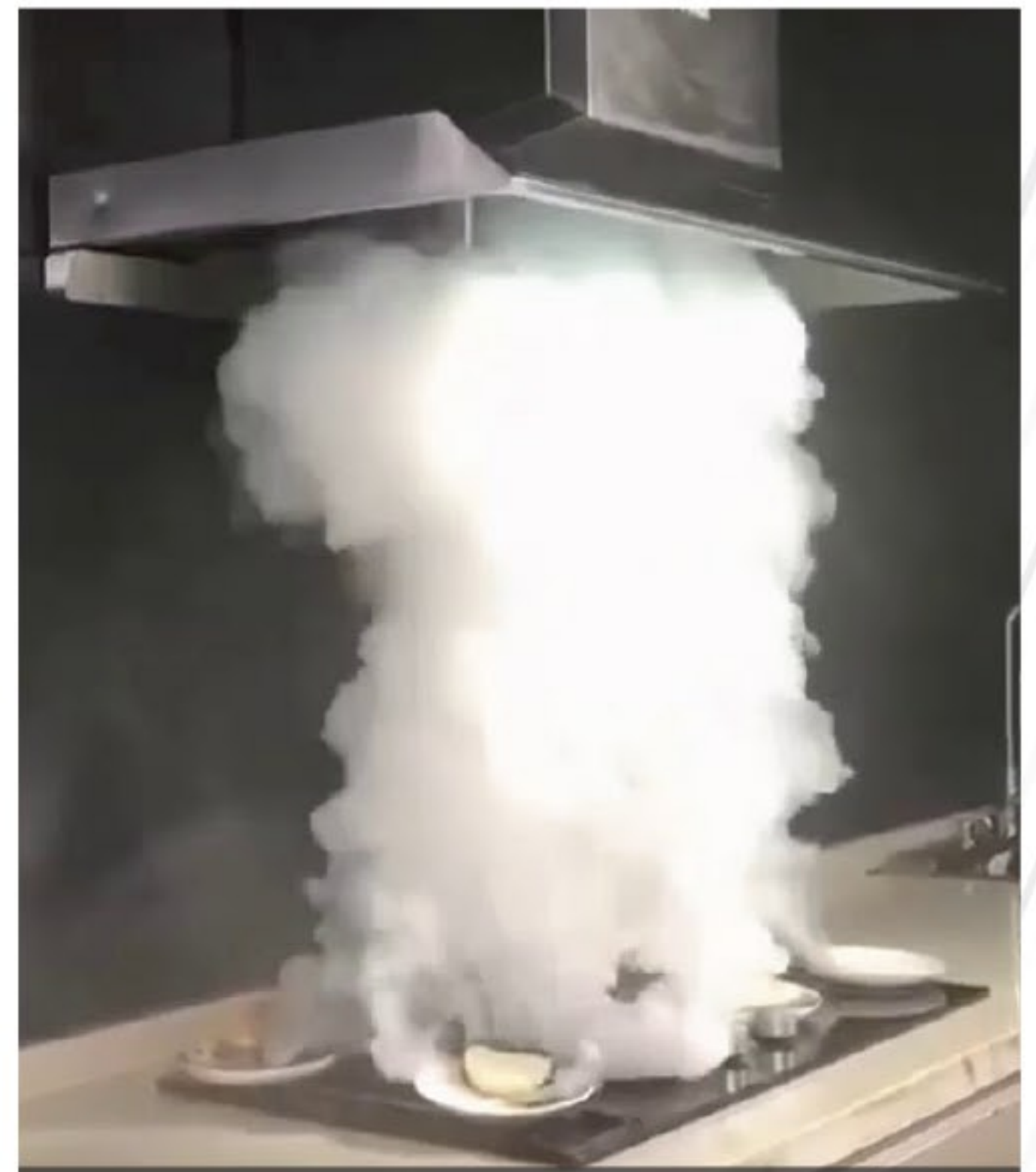
Smoke Clearance Test
